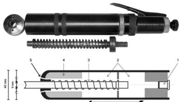
FIG. 1—Scheme of a captive-bolt gun (1, Blanc cartridge; 2, chamber; 3, metal bolt with a withdrawal spring; 4, boundary; 5, diverging smoke conduits).
